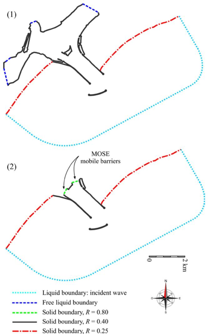
Figure 7. Domain contours. (1) MOSE barriers off and (2) domain limitation imposed by MOSE mobile barriers.
