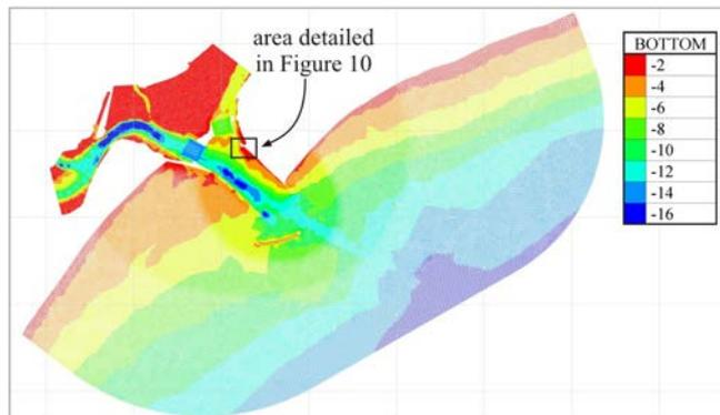
Figure 9. Bathymetry and computational grid (case i.1).
