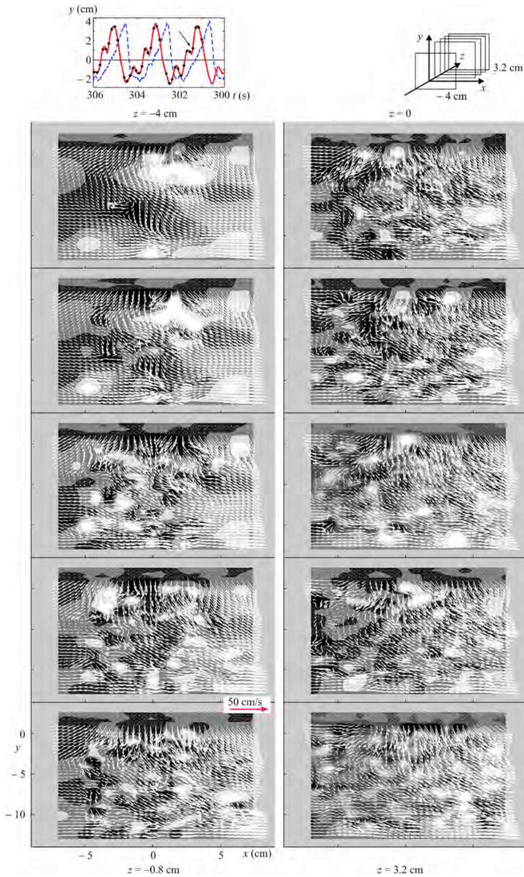
Figure Appendix A.1. Instantaneous velocity vectors (only cross-shore and vertical components) for Experiment 6b, fourth phase, first wave cycle.
